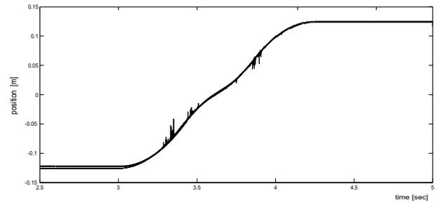
Figure 5: Reference signal and actual cart position
