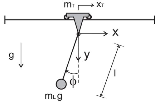
Figure 1: Cart-pendulum scheme
