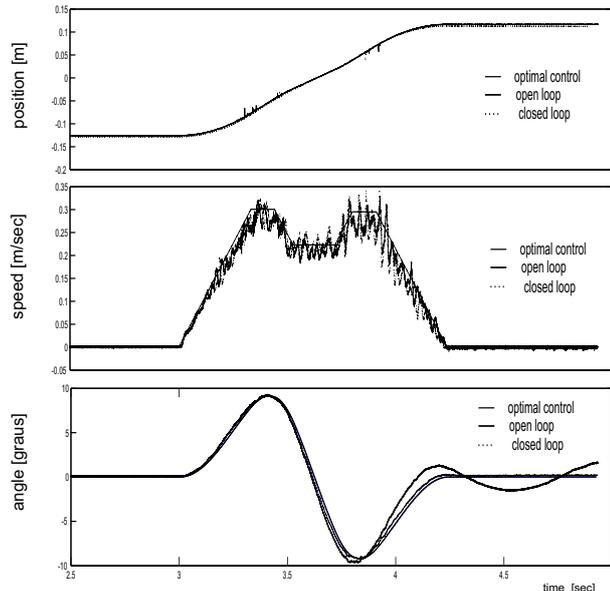
Figure 14: Cart positions, cart speed and pendulum angle for  $l=0.15$  m, closed loop and open loop
