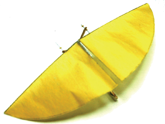
Figure 8: Flapping Robot without Tail Plane
