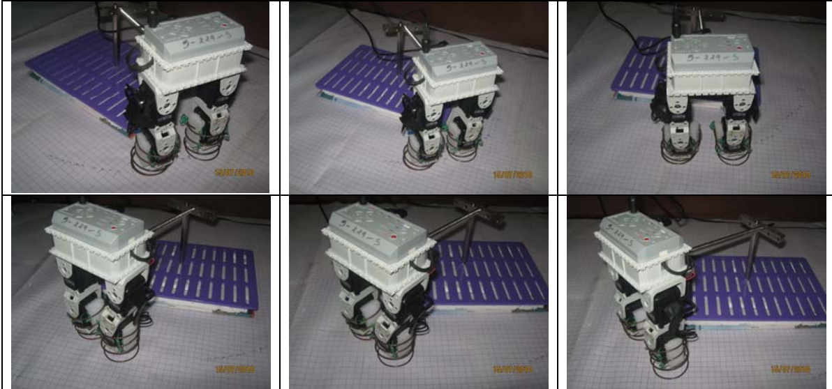
Fig. 10 Snapshots of sagittal plane locomotion of flexible legged walking robot
