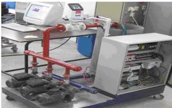
Figure 2: experimental test bench of the pumping unit
