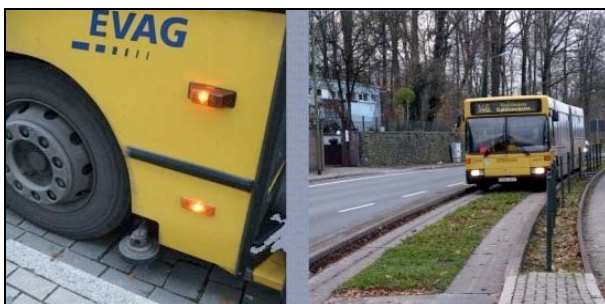
Figure 11: Curb guided system in Essen
