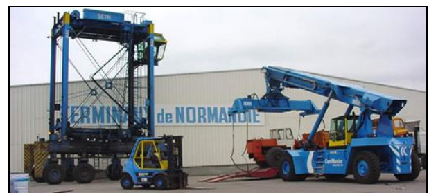
Figure 5: straddle carrier, forklift truck and a reach stacker used in the Terminal de Normandie (source: http://www.t-n.fr ).
