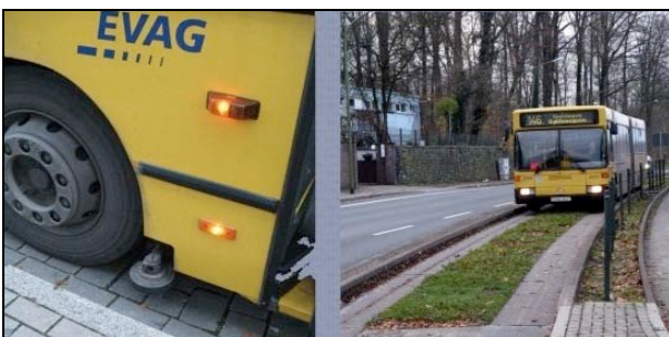
Figure 11: Curb guided system in Essen
