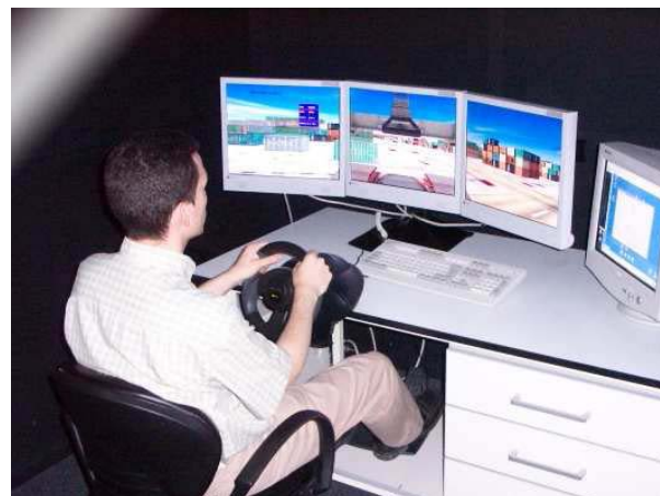
Figure 4: A desktop configuration, with several displays and conventional game devices as controls
