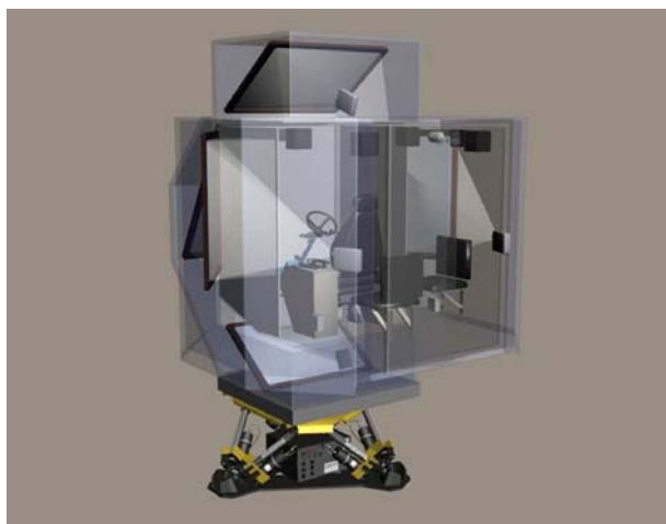
Figure 6: A CAD view of a Fully Immersive simulation system
