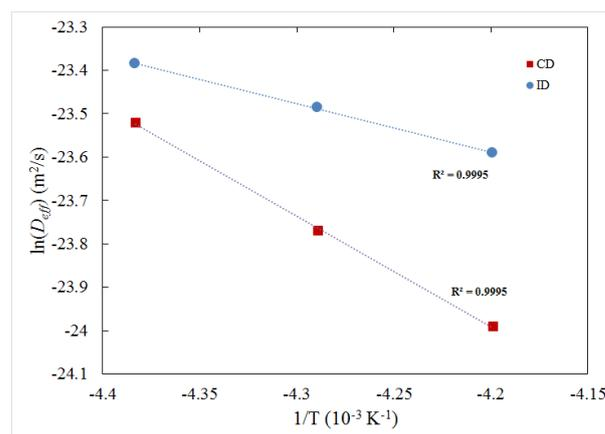
Figure 5: Comparison of the Activation Energy of Samples Dried by Continuous Drying (CD) and Intermittent Drying (ID).
