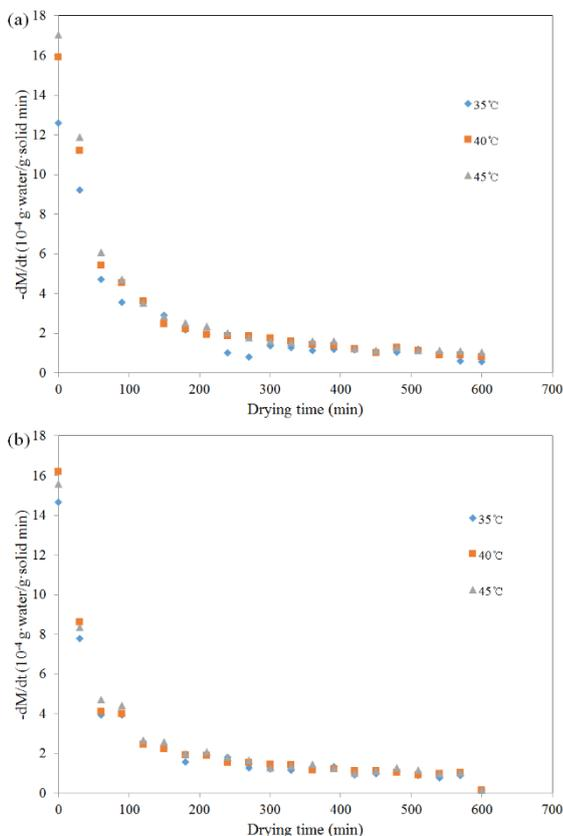
Figure 3: Effect of Drying Temperature on the Changes of Drying Rate Using (a) Continuous Drying and (b) Intermittent Drying.
