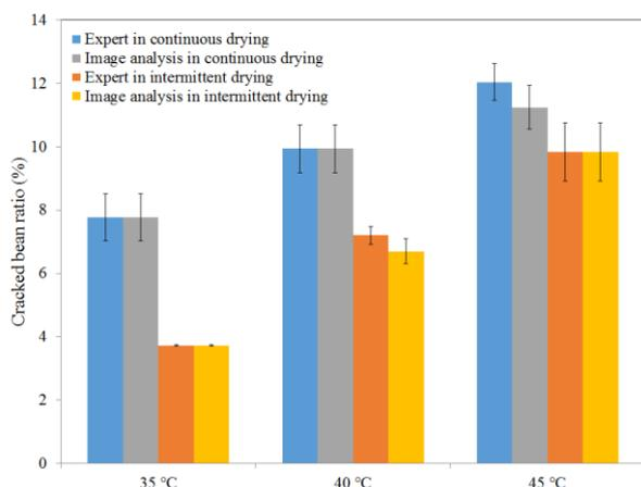
Figure 4: Effect of Drying Temperature on the Cracked Grain Ratio at the Target Moisture Content of 7.7%.
