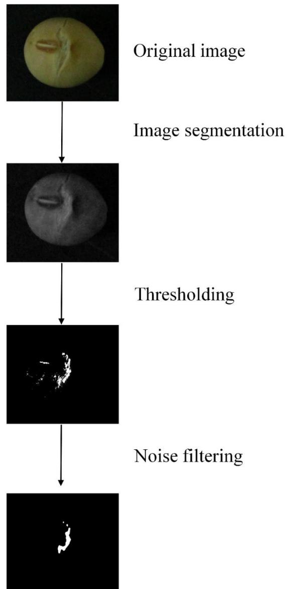
Figure 1: The Overall Procedure for Image Analysis of Soybean.
