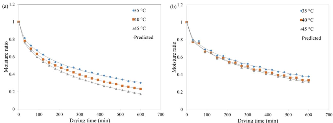
Figure 2: Changes of Moisture Ratio of the Soybean Upon the Drying Temperature Using (a) Continuous Drying and (b) Intermittent Drying.
