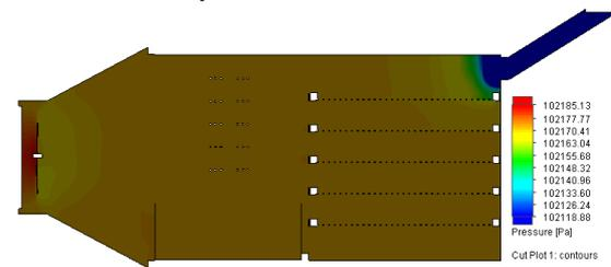
Figure 5: Pressure Profile of the Hot Air in the CECH Dryer
