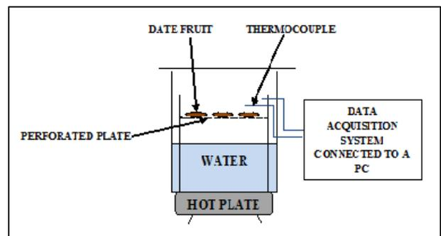
Figure 1: Laboratory Experimental System Designed for Dates Hydration
