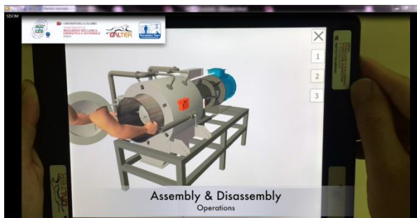
Figure 4: A sample of 3D animation for maintenance procedures
