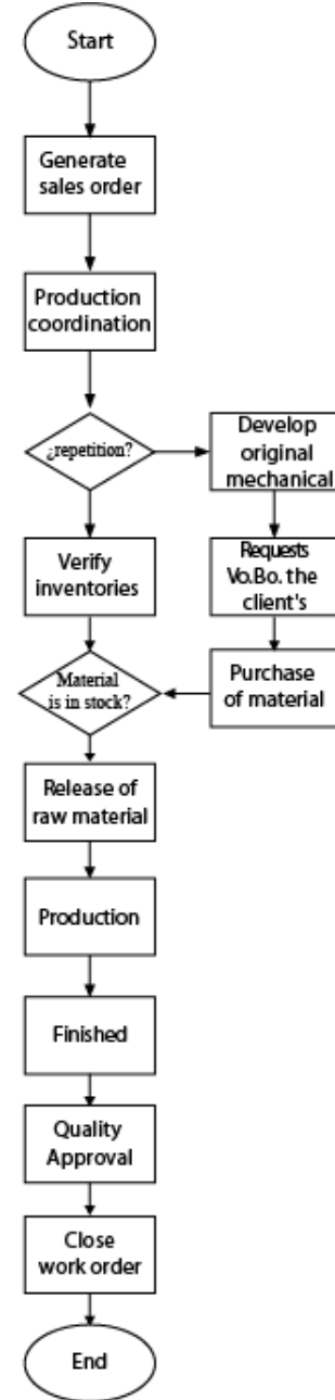
Image 5. General Process Diagram For Printing Of Folding Packaging. Own elaboration.
