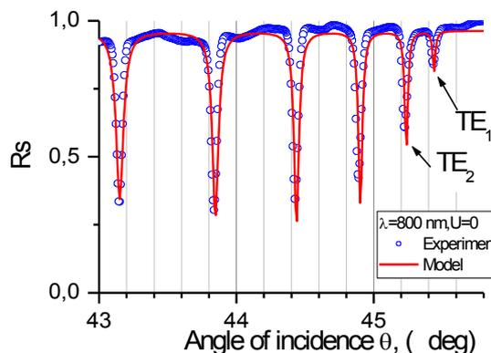
Figure 3: The Angular Reflection Spectrum  $R_s(\theta)$  of six layers sample in the case of TE (S) polarization of the incident radiation. The solid line is the modeling, the circles are the experiment. The wavelength is  $\lambda = 800 \text{ nm}$ . Sample S1
