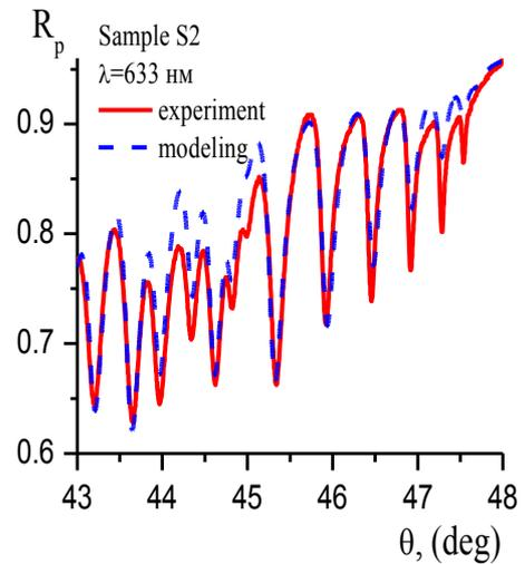
Figure 4. The measured and calculated angular reflection spectrum of  $R_p(\theta)$  at a wavelength of 633 nm for sample S2.
