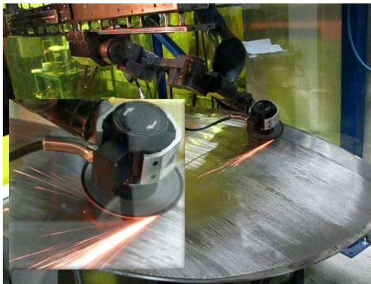
Fig. 3 Robotic grinding of a Francis turbine runner blade (Sabourin et al., 2010).
