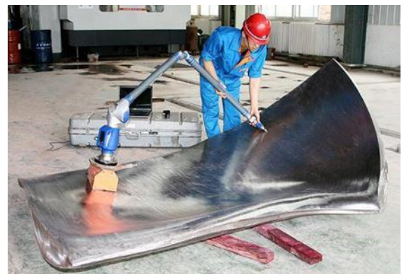
(b) Inspection of a raw blade after machining
