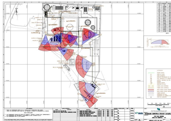
Figure 4. Plant Fire System Coverage
