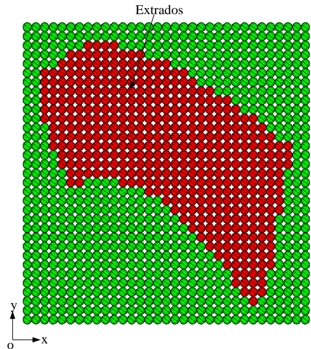
Fig. 13 Upper array of the pins of the pressing process
