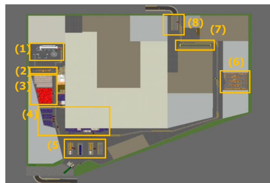
Figure 1: 2D SIMIO Model - Layout. (1) Packaging Line, (2) Line Temporary Stock Area, (3) Warehouse and cellar belonging to line, (4) "Others" Warehouse, (5) Main Loading and Unloading Area, (6) Raw Materials Warehouse, (7) Secondary Temporary Stock Area, (8) Secondary Loading and Unloading Area
