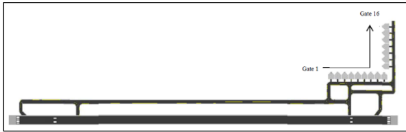
Figure 5: Configuration L-shaped stand with partial parallel taxiway
