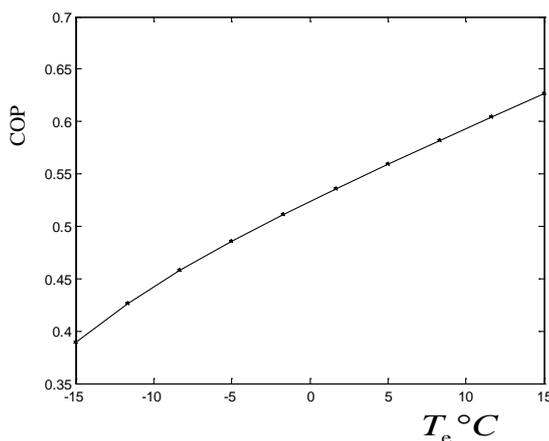
Figure 9: Variation of COP with different refrigerating temperatures
