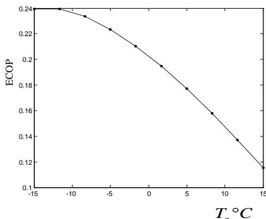
Figure 10: Variation of ECOP with different refrigerating temperatures
