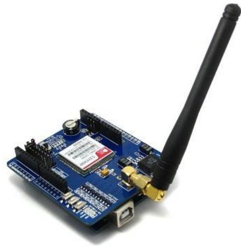
Figure 6: SIM900 GSM/GPRS (IteadStudio, 2012)
