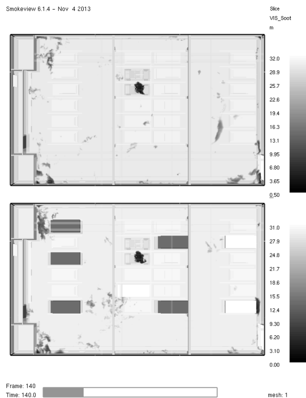
Figure 11: Fire scenarios "full" and "full-8van" and D1 configuration. Creation of smoke clusters in vans proximity at t = 140s.
