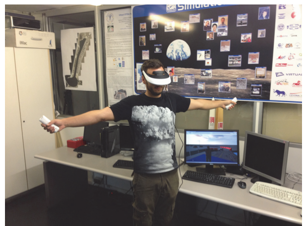
Figure 5: the real operator controlling the avatar through a motion controller and experiencing the virtual environment through a mounted head display
