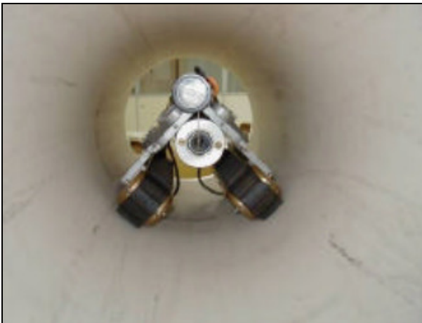
Figure 2: Example Robot for Internal Inspection of pipelines with treadmills
