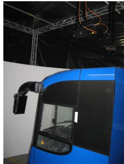
Fig. 2. Simulator with a cylindrical screen - visible cabin, cylindrical screen and projection system.
