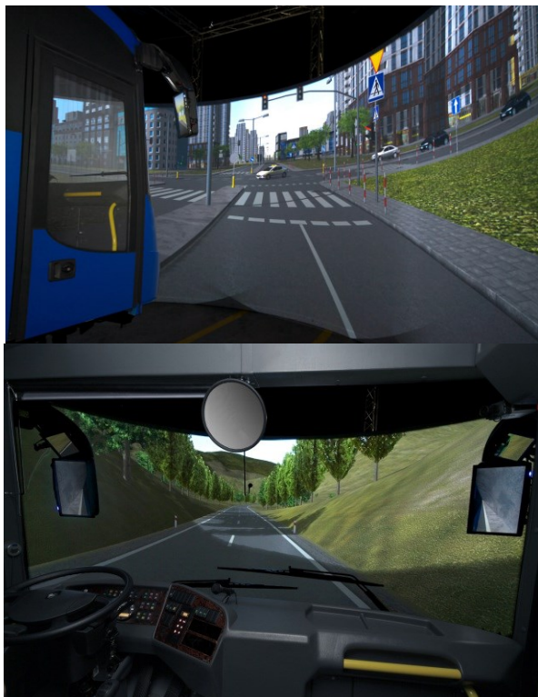
Fig. 1. Simulator with a cylindrical screen - a view of the cabin and the screen with displayed image, from outside and from inside of the cabin.
