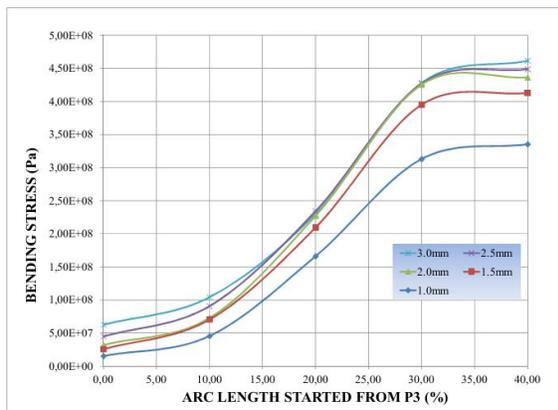
Figure 8: Stress distribution for various plate thicknesses
