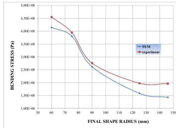
Figure 10: Stress distribution for various final shape radius.
