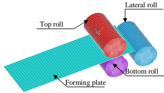
Figure 3: FEM model of roll bending process
