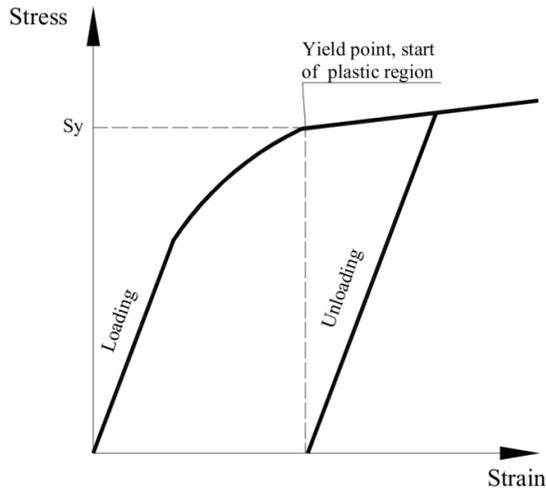
Figure 2: Types of loadings in roll bending process
