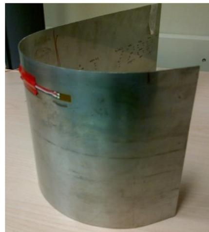
Figure 11: Workpiece after roll bending process
