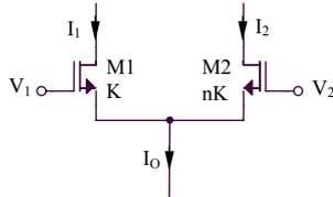
Figure 3: Asymmetrical differential structure
