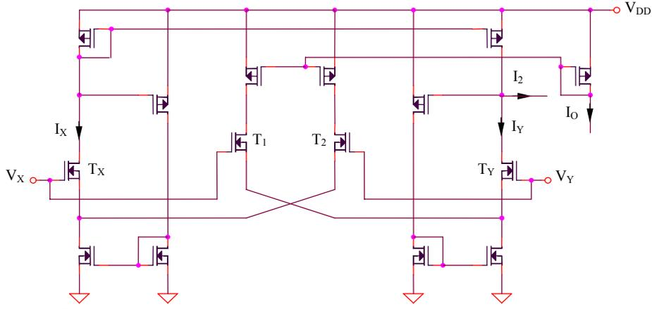
Figure 2: The linearized differential structure
