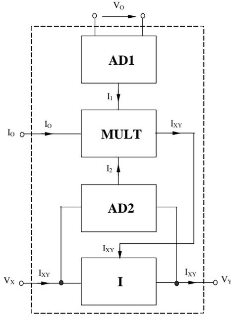
Figure 1: The block diagram of the active resistor
