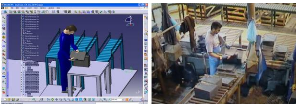
Figure 12: Splitting with Turning. The part is lifted and turned to be split again.
