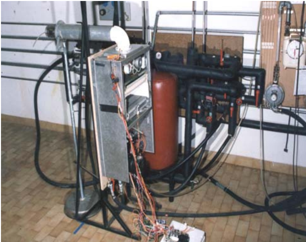
Figure 3: The prototype of high efficiency domestic combined boiler.
