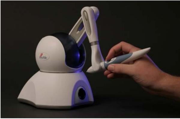
Figure 3 – Phantom Omni haptic device
