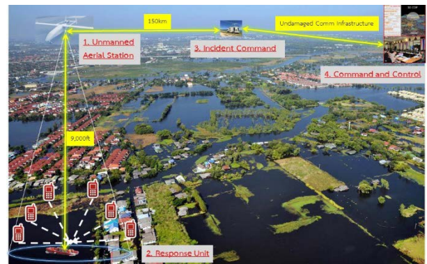
Figure 1: An operational view of the mesh communication backbone
