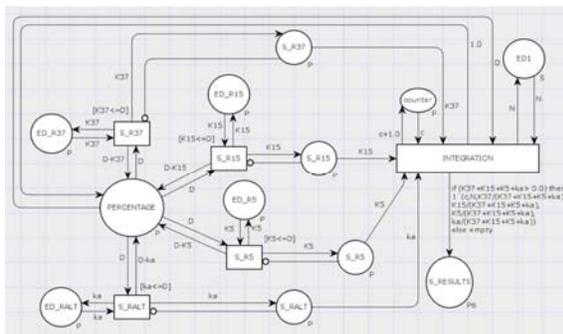
Figure 9: CPN Model for Simulation of Displacement Flows
