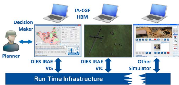
Figure 1: DIES IRAE Architecture
