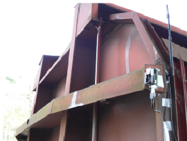
Figure 8: MicaZ network master outside the car
